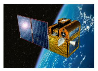
Fig. 1: Artist view of PICARD microsatellite, 60x60x80 cm3 in size. Shown are the 3 instruments of the payload: SODISM, telescope and guiding, right, SOVAP, differential radiometer, center, and PREMOS (flux monitors) left, near the solar panels. In the back, one can see the electronics box supporting two S-band antennae and a solar pointer (acquisition maneuvers).
